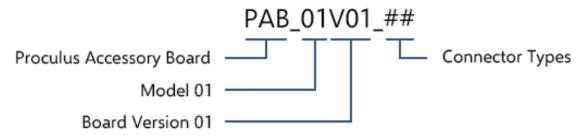
You can order PAB\_01 in any configuration of pre-assembled connector types. The following table lists part numbers for the most common (and readily available) configurations:
