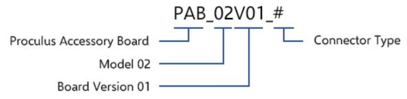
You can order PAB\_02 in any configuration of pre-assembled connector types. The following table lists part numbers all available configurations:
