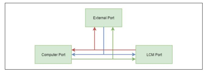
For example, if the computer sends a message to the board (through the **Computer Port**), the message is sent to the **External Port** and to the **LCM Port**.
