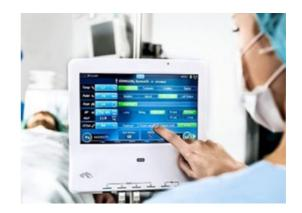
Operating a display whilst wearing gloves is common in the medical world. We can optimize the Capacitive Touchscreen (PCAP) to support gesture/multi-touch functionality with different glove types.
